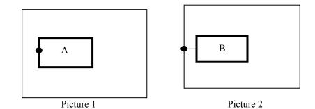
As picture 1, the outer is square steel plate and the inside rectangle is the workpiece to be cut. Assuming that it is to cut the work piece from point A and the steel plate is of thick materials; then, it will cost a lot of time to perforate. However, if it is to cut from the edge of steel plate (point B), the time of preheating perforating may be saved. Detailed operations are as follows:
