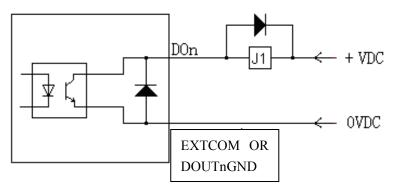
EXTCOM is connected to the negative end of internal power supply, and the output signal is connected to the relevant terminal.
