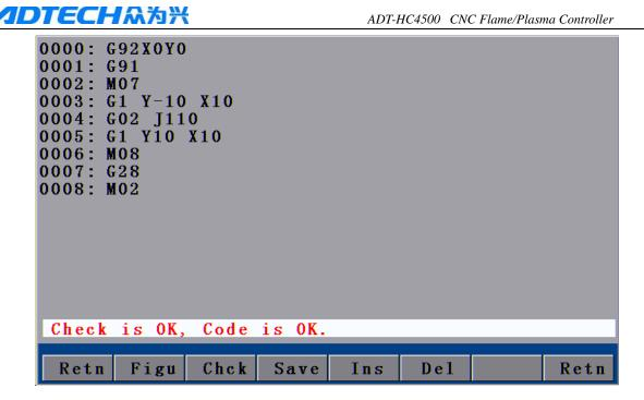
Picture 3.2.1.2 Error code detection interface
